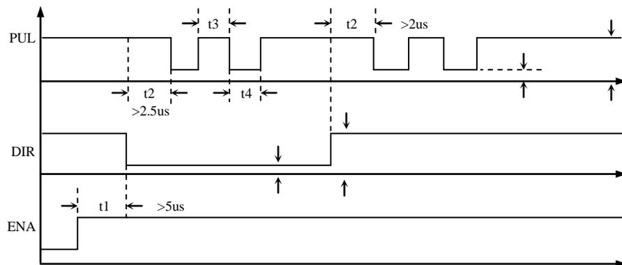
Figure 10: Sequence chart of control signals
