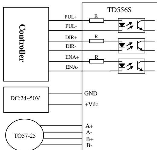
Figure 9 TD556S Typical connection
