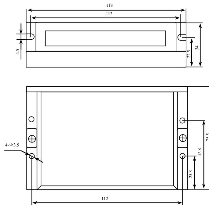
Figure 1: Mechanical specifications
