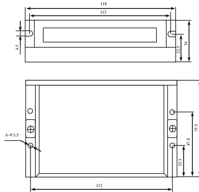
Figure 1: Mechanical specifications
