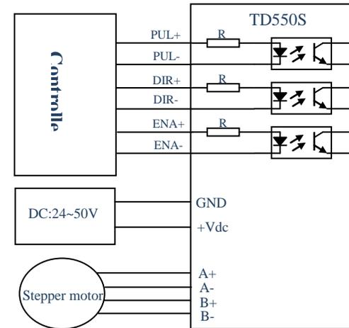
Figure 9 TD550S Typical connection
