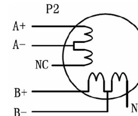
Figure 5: 6-lead motor half coil (higher speed) connections
